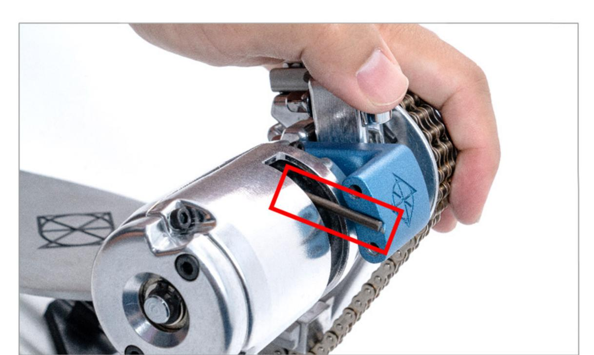
Tighten the 2 screws on the blue spring holder cap with 3mm Hex L rod.
