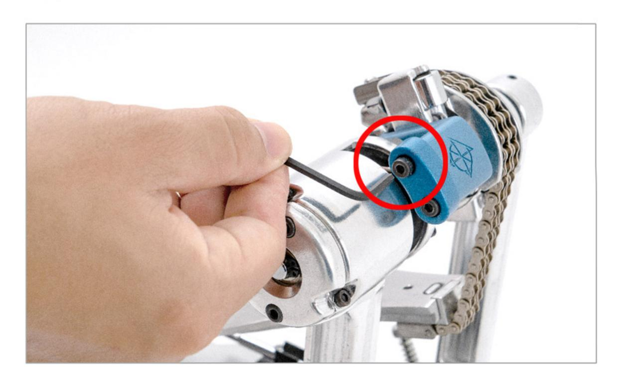
Make sure the cap is equally tightened on both ends.
