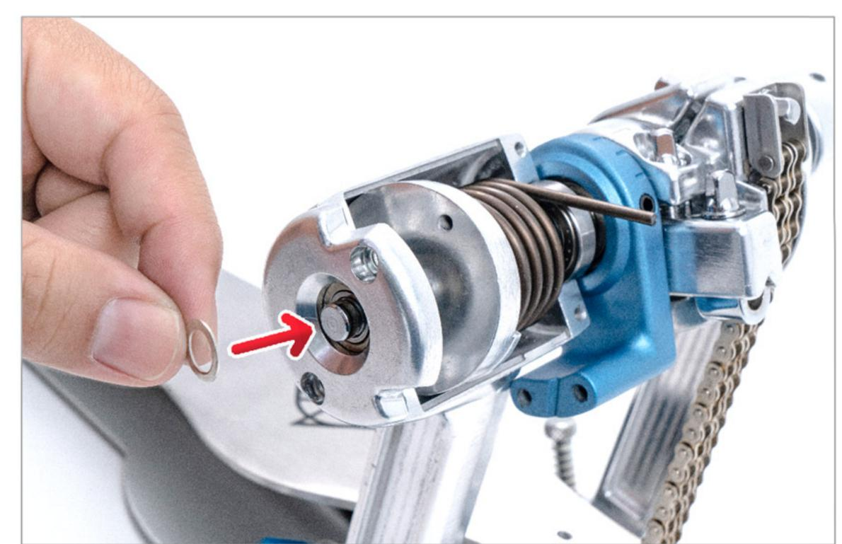
Put the C-clip back onto the connecting post with pliers.
